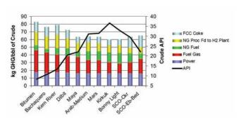
Figure 5-15 GHG emissions from energy sources used to refine crude, SCO, bitumen, or dilbit 184.
